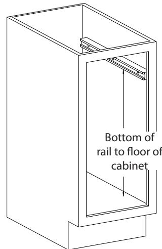
**8)** Install second rail on opposite side of cabinet per steps 5-6 at height location from step 7.
