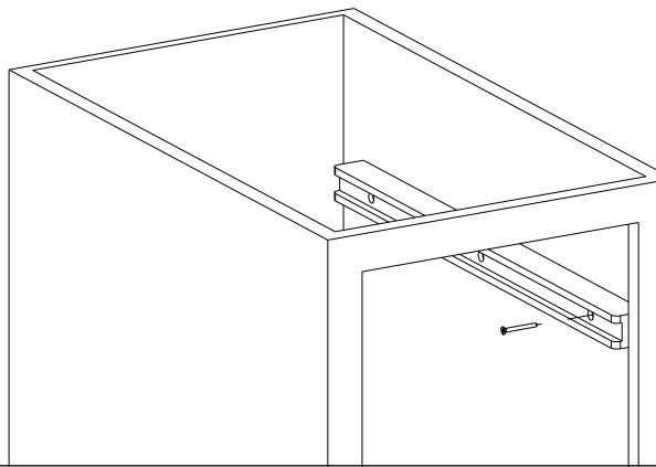
**6)** Make sure rail is level, then secure to cabinet with screws at remaining hole locations.
