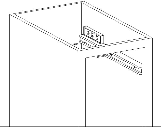
**7)** Measure from floor of cabinet to bottom of installed rail.
